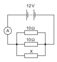
The battery has e.m.f. 12 V and negligible internal resistance. The ammeter reading is 3.2 A.
